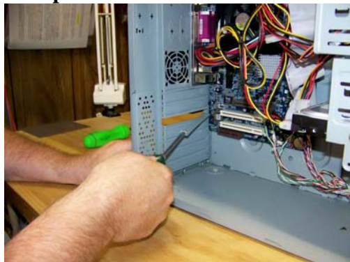
Open slot on back of computer to install card
