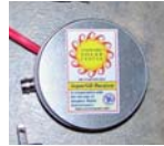
A PreAmp to raise very small signals to a level can be captured by a PC sound card.
